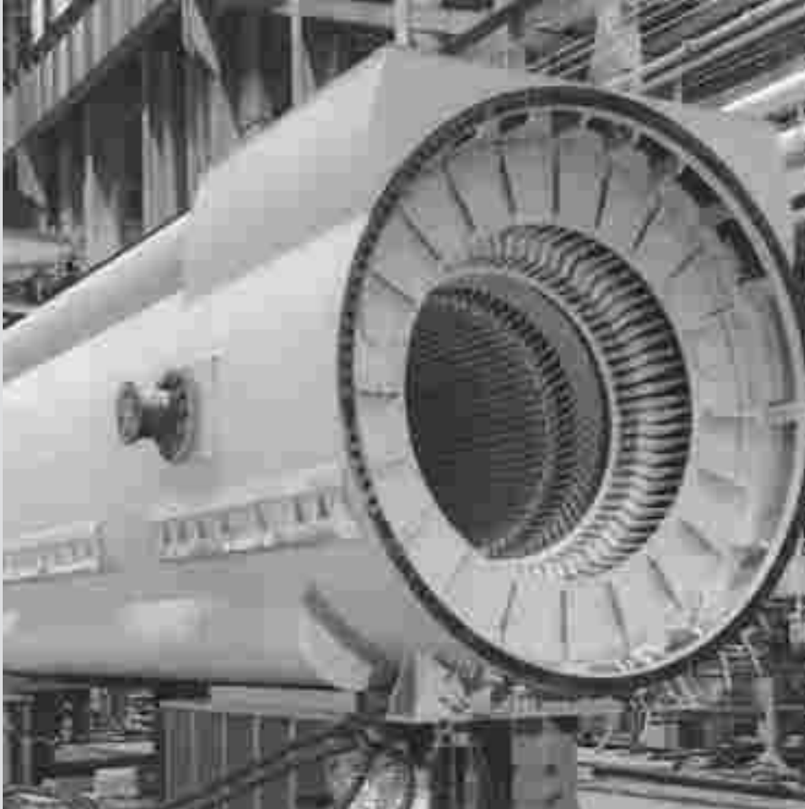
Generator stator showing completed windings for a 757-MVA, 3600-RPM, 60-Hz synchronous generator (Courtesy of General Electric.)
