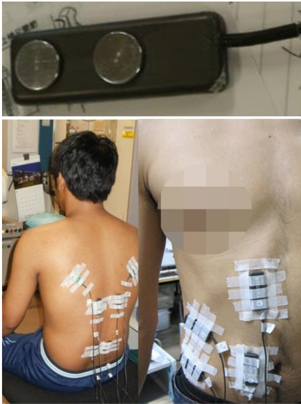
Figure 3. sEMG Ag/AgCl bipolar electrode (upper) and sEMG electrodes attachment onto the skin surface to measure back and abdominal muscles activation (lower)
